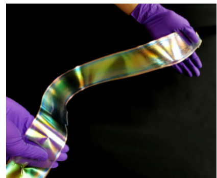
This shiny ribbon contains tiny arrangements of cellulose that reflect light in specific ways to give the material its color.
